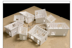
Model: roof structure.
