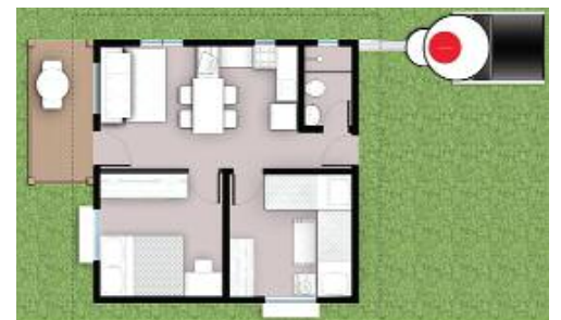
Changes according to conditions recommended by the Brazilian standard BR 15220-3, with insertion of the tower to the house.
