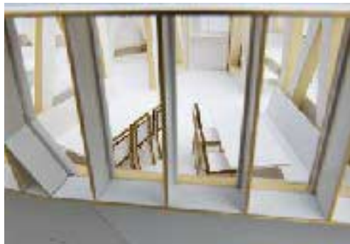
The staircase plays an important role in the use of passive solar energy; at the same time it acts as the air circulation network for the upper floors.
