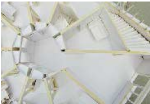
The staircase plays an important role in the use of passive solar energy; at the same time it acts as the air circulation network for the upper floors.
