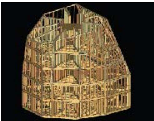
The “light-weight” wooden structure is made of computer-aided prefabricated elements.
